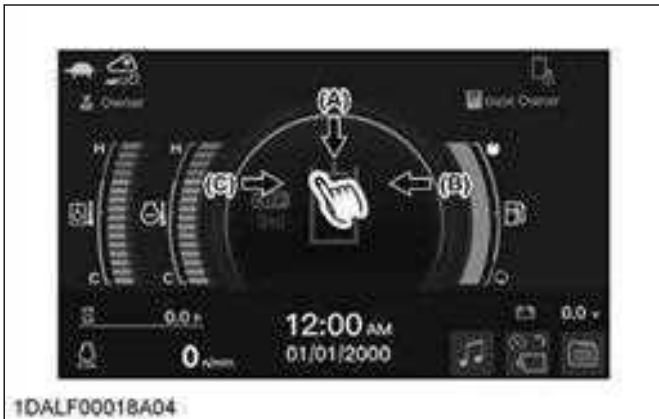
(A) To rearview camera screen (C) To audio screen (B) To memo screen
